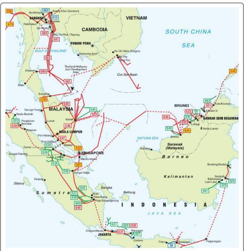
**Fig. 7** Southeast Asia pipeline map: crude oil (petroleum) pipelines - natural gas pipelines - product pipelines (Information Technology Associates 2008)
