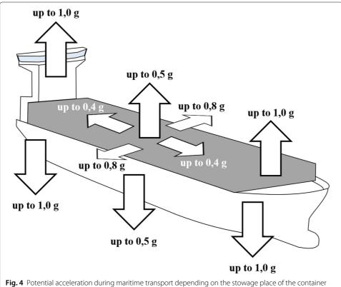
**Fig. 4** Potential acceleration during maritime transport depending on the stowage place of the container (based on Hapag-Lloyd Container Line – Special Cargo Department (2005), p. 5)
