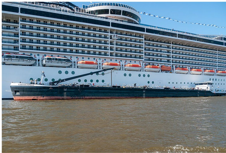
Fig. 7 Bunkering for a cruise vessel (source: Wikimedia Commons the image is used under a CC BY-SA 4.0 license)
